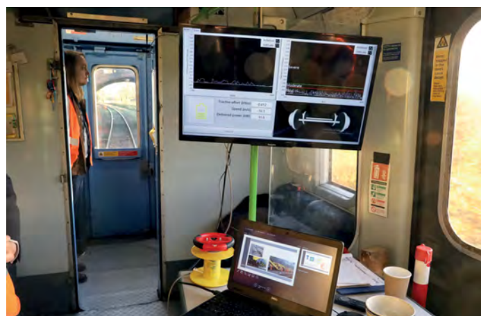
Monitoring: kit inside the D train following the movement of the ActiWheel.
