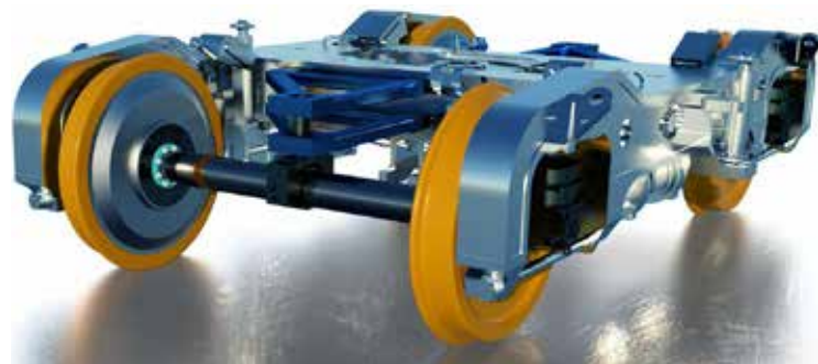
Axle with ActiWheels and frame.
