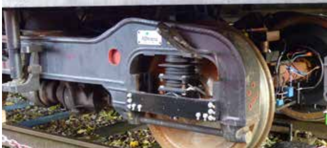
Modified primary suspension.
